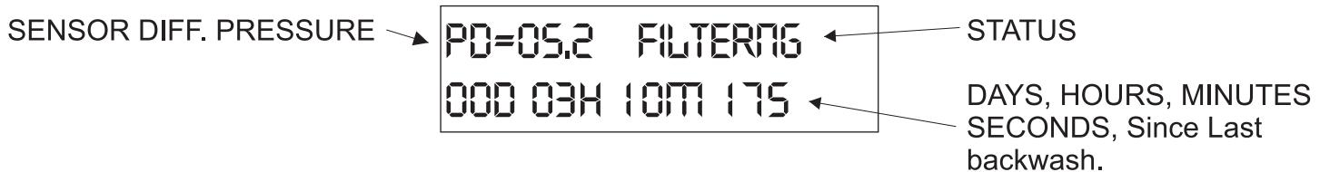
**P.D. DIFFERENTIAL SETTING:** Use this setting to set the trigger point for the sensor gauge based on the SENSOR/GAUGE TYPE function. If the function is set for "P.D. GAUGE" then this display will show: "SET DIFFERENTIAL PSI ON GAUGE" and no adjustable parameter is available. If the SENSOR/GAUGE TYPE function is set for "SENSOR", then a differential trigger setting will be available for adjustment. Press SELECT, +, and - to set the backwash trigger point of the sensor.
