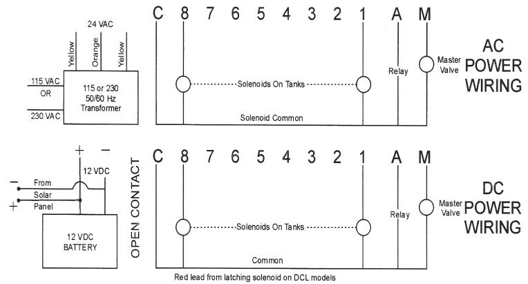
DO NOT USE TRANSFORMER AND WIRE + - 12 VDC TO FIRST TWO TERMINALS. DO NOT USE THIRD TERMINAL.
